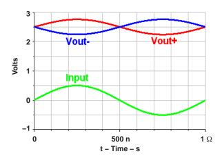
Figure 3-3. Output of an AC-Coupled, Single-Supply Application
